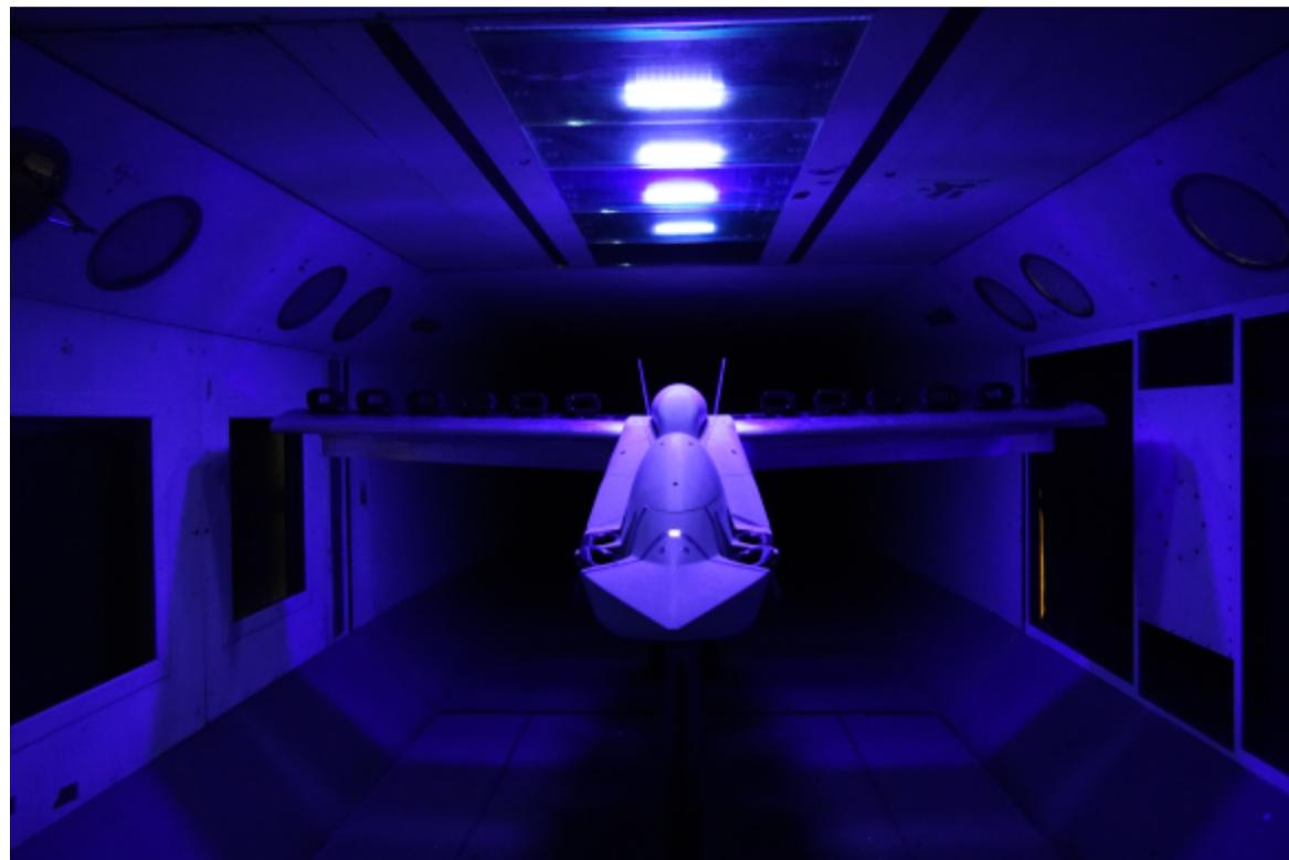
Wind tunnel model has fluidic thrusters over the wing for lift augmentation and embedded in the fuselage for vertical thrust.
